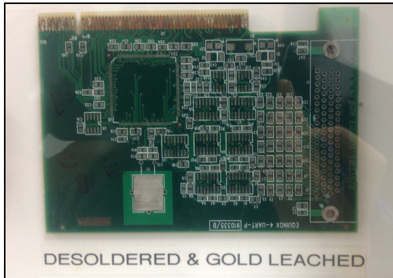
Figure 5. Desoldered and Gold Leached Printed Wiring Board
